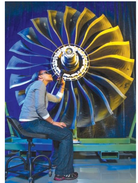
Final assembly of the first PW1100G engine, the model that will power the A320neo.
